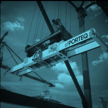
Our lightweight energy saving spreaders share components from our RTG/RMG and STS spreader products. This unique spreader is primarily intended for applications where weight is of greater significance than hoist speeds and top lifting capacity. They are designed to handle containers of 20 to 45 feet with ISO twistlocks. The TEESH+ is the only existing expandable twin under 10 tonnes tare weight.
