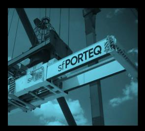
Our mobile harbor spreaders (MHC) serve exacting demands in terms of robustness and versatility. They are designed to handle containers sized from 20 to 45 feet with ISO twistlocks. Our MHC spreaders are electric hydraulic, based on a proven technology to give the spreaders the required strength and endurance for continuous operation. Throughout the design process, special attention has been given to maximising up-time and making maintenance as simple as possible.
