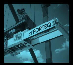
This platform is built for the most environmentally challenging segment within container handling. With a robust yet simple design, and carefully selected components, this single lift spreader is purpose-built for the harsh environment of ship-to-shore operations. It is designed to handle containers sized from 20 to 45 feet with ISO twistlocks.
