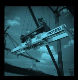
Our lightweight energy saving spreaders share components from our RTG/RMG and STS spreader products. This unique spreader is primarily intended for applications where weight is of greater significance than hoist speeds and top lifting capacity. They are designed to handle containers of 20 to 45 feet with ISO twistlocks. The TEESH+ is the only existing expandable twin under 10 tonnes tare weight.
